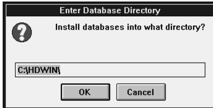
For multiuser access, the databases must be installed to a network directory. The file server should have at least 50 MB of available disk space.
